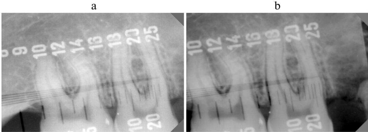
Fig. 2. Photographs of mandible taken using apparatus with focal spot diameters of 0.7 mm (a) and 0.2 mm (b).
